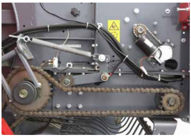
TRANSMISSION DIVIDED ON TWO SIDES
