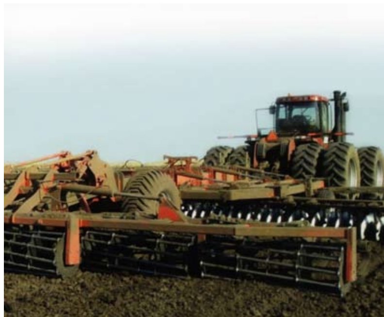
Rullo GABBIA Ø 600 - 12 tubi CAGE roller Ø 600 - 12 tubes Rouleau CAGE Ø 600 - 12 tubi
