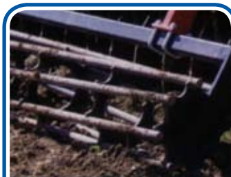
Rullo Gabbia Ø 540 - 11 tubi CAGE roller Ø 540 - 11 tubes Rouleau CAGE Ø 540 - 11 tubes
